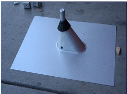
4) Attach the standoff shaft and tighten it onto the base stud with channel locks. Set the flashing by sliding it over the standoff and directly applying it to the roof surface, using all necessary sealants and attachment methods for flashing. Slide Rubber Rain Collar over the standoff shaft to cover top of flashing.
