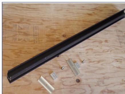
1) Construct High Tilt Tool using a length of SnapNrack rail cut to the dimensions of the module(s) being installed, two 4" lengths of Rail Cover with 3/8" holes drilled in the center of each, two channel nuts, and two 5/16" bolts.
