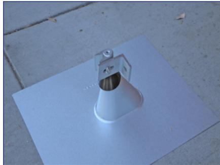
5) Slide the standoff clamp and L Foot onto the standoff shaft, adjust it to the desired height, and tighten hardware to 10-16 ft-lbs.
