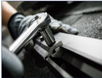
4) Use a socket wrench to tighten splice bolts, torque silver hardware to 10-16 ft-lbs and black hardware to 8-10 ft-lbs.
