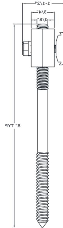
Dimensioned Hanger Bolt Clamp Assembly
